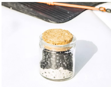
Bureo recycles the nets down into a raw material in the form of pellets.
